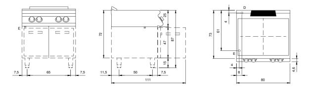
E: Electric power D: Drain for water
